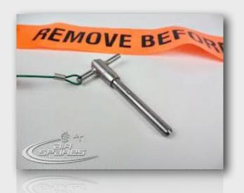
It says this occurred through a combination of deficiencies in the operator's task-card system, inadequate handover between engineering shifts, and the distraction of an engineer – who had noticed the rig pin's absence and, concerned about possibly being injured, had taken an overdue break.
